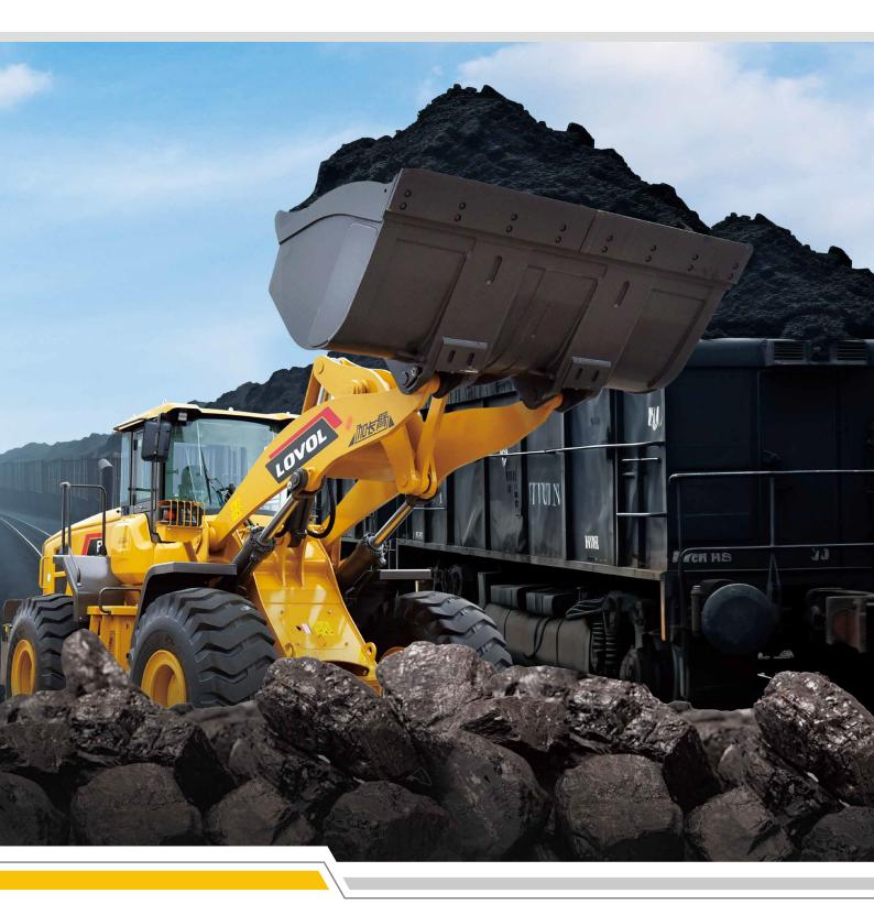
Engine Model Rated Power Operating Weight Bucket Capacity Max. Breakout Force WEICHAI WP10G240E341 178kW 20590kg 4.0m<sup>3</sup> 180kN
