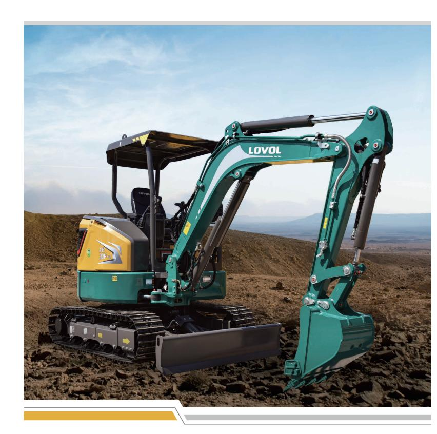
Rated Power 22.2kW/2400rpm
